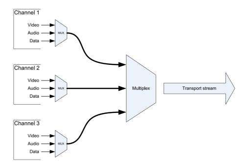
Figure 2.1: Multiplexing of several programs into a single transport stream in MPEG-2.
