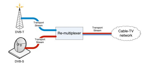
Figure 2.3: Re-multiplexing of channels
